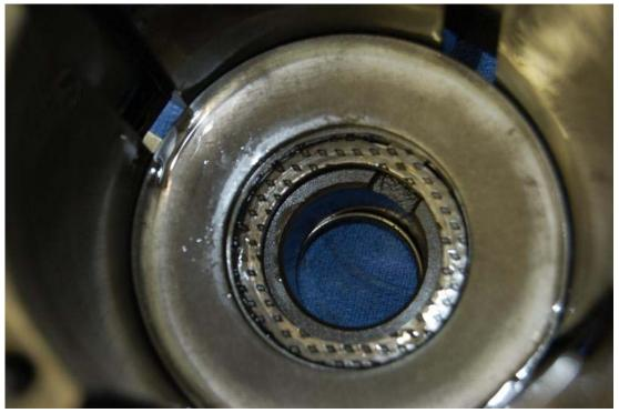
Step 11. Install clutch discs. Adjacent to each disc is a dog ring friction disc. These should be flipped to provide a fresh friction surface.
