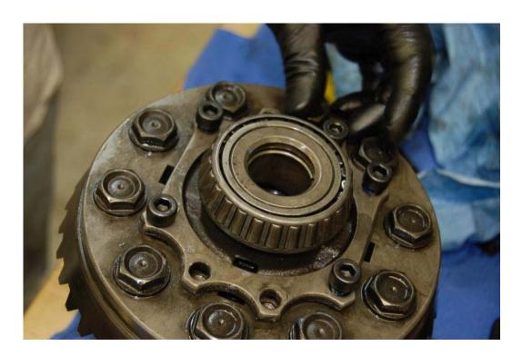
Step 13. Replace the internal assembly into the case. This can be done alone, however having a second person may help. You will need to hold the assembly and rotate in input shaft to mesh it with the ring gear. This will need to be done as the outer bearing race covers are placed back into the sides of the case. Replace the 13 mm hex head bolts and snug down.
