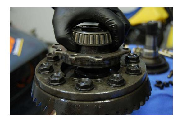
Step 10. Remove the internal parts – friction surfaces, clutch discs, gear clusters. One of the clutch discs will be one side of the center gear cluster, the other one on the other side. As you remove the parts, it may be helpful to stack them as you remove them so you can reinstall in the same in order.
