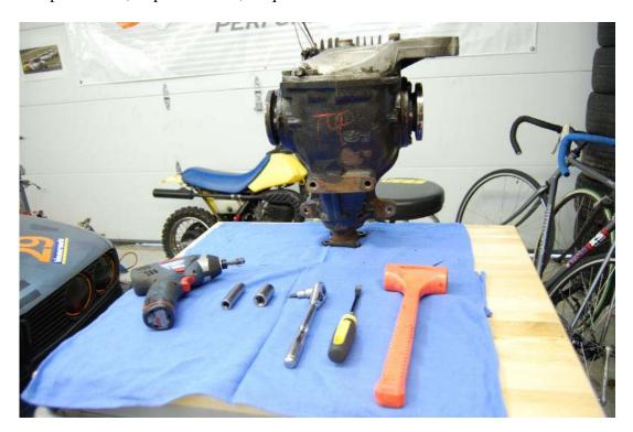
Step 5. Remove the rear cover (17 mm hex head bolts).
