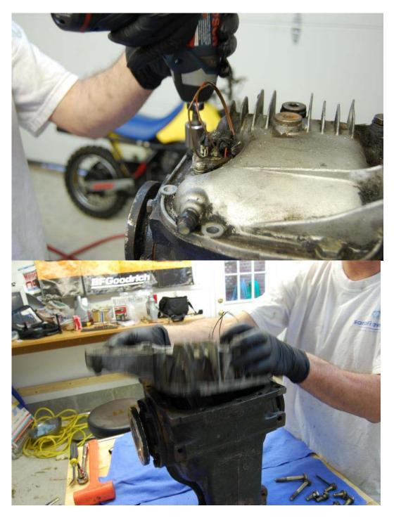
Step 6. Remove the output shafts. These should just pop out with a little tugging, but you may need to use a pry bar to get them out. They are splinned shafts and held in by a small circlip.
