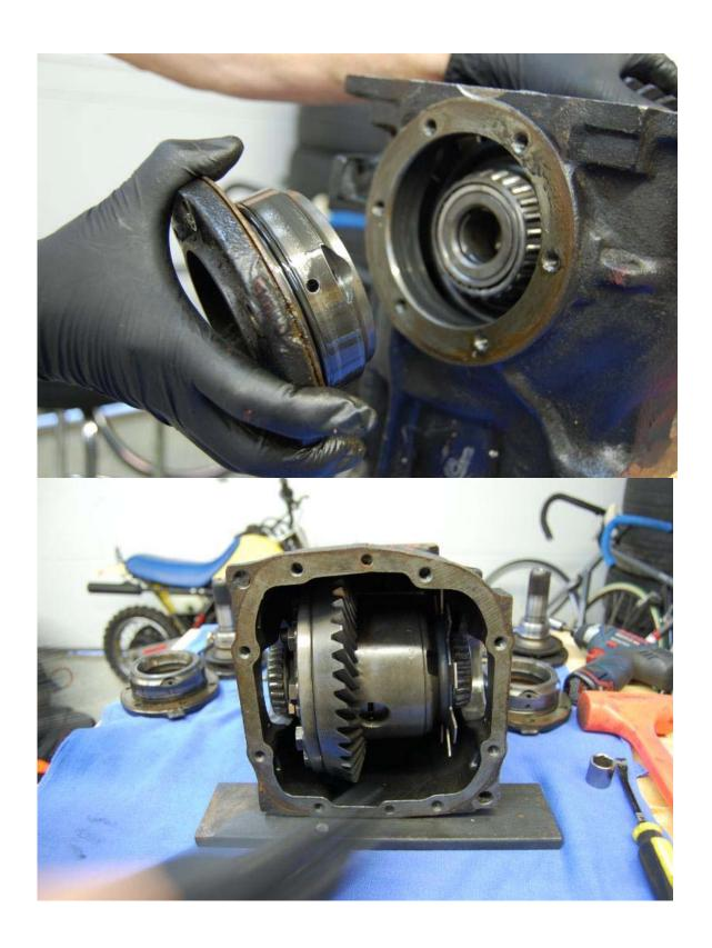
Step 8. Pull the limited slip assembly from the housing. Stand it on end so that the bearing with the cover plate side is facing up. Remove the 6 mm half-height socket head screws. Be careful as you may strip out the heads (as we did).
