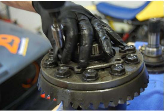
Step 9. Remove the cover plate. This may require to gentle prying with a pry bar or screw driver. Move around prying small amounts around the surface. This will require some patience. As the cover is released pay careful attention the washers underneath. These will need to be reinstalled in the same order. In addition, there is a larger convex washer. This will need to be reinstalled later in the same direction.
